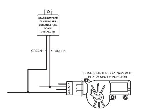
The emulator AEB429 only draws and does not interrupt the wire of the signal on which it works; in this way, during the gasoline the emulator has not influence on the car original system; this applies also in case of failure to the GAS system, thus allowing the user to drive the car with gasoline and reach a service point for checking.
