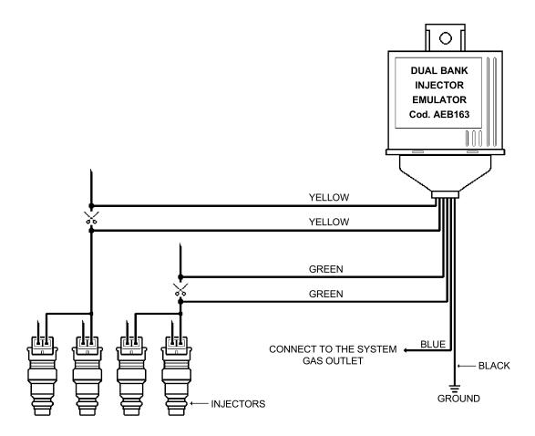
On the AEB163 emulator it is possible to adjust the overlapping time that is calibrated when sold with an optimal time of approx. 0,4 seconds for most cars.
