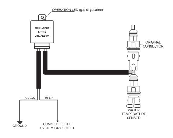
The AEB444 emulator switches on during the gas running and switches off during the gasoline running, thus automatically resetting the connections to the car original electrical system; this applies also in case of failure, thus allowing the user to drive the car with gasoline and reach a service point for checking.
