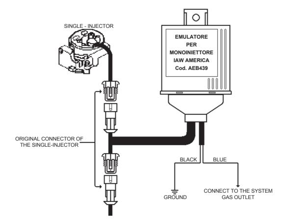
The AEB439 emulator is equipped with a trimmer to adjust the overlapping time, from  $0 \div 1$  second approx., and with two switches to select the type of emulation. When sold, the emulator is set up with an optimal overlapping time of approx. 0,4 seconds for most cars and with the correct emulation for the above - mentioned cars; for this reason, the button must not be touched.
