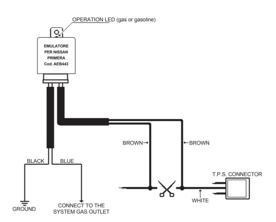
The AEB443 emulator switches on during the gas running and switches off during the gasoline running, thus automatically resetting the connections to the car original electrical system; this applies also in case of failure, thus allowing the user to drive the car with gasoline and reach a service point for checking.
