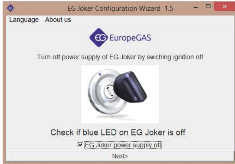
Fig. 3: Turning EG Joker power supply off.
